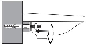
5.Screw a metal nut onto each fixing bolt to secure the basin.Caution:Do not over –tighten,as this may damage the ceramic
