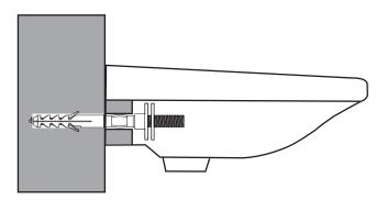
4.Place the basin in position against the wall, iocating the fixing bolts through the holes in the rear of the basin.Push a plastic washer onto each fixing bolt
