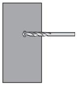
1.Drill two holes in the required position on the wall using a 14mm masonry drill bit.to a depth of 75mm
